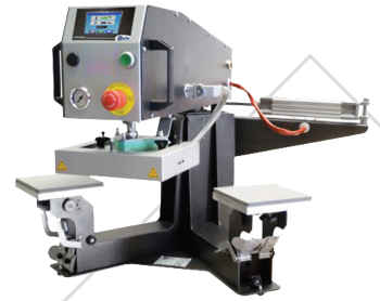
DUPLEX AUTO MINI PLA T Plate : Flat 16x16cm Automatic Translation Touch Screen
